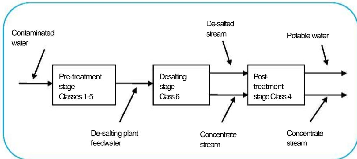
Figure 1: Water treatment process and classes of contaminants
