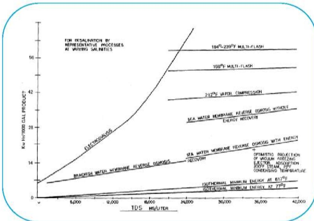
Figure 2: Energy efficiency (kWh/1000 gal) of representative desalination technologies as a function of total dissolved salts (mg/L)
